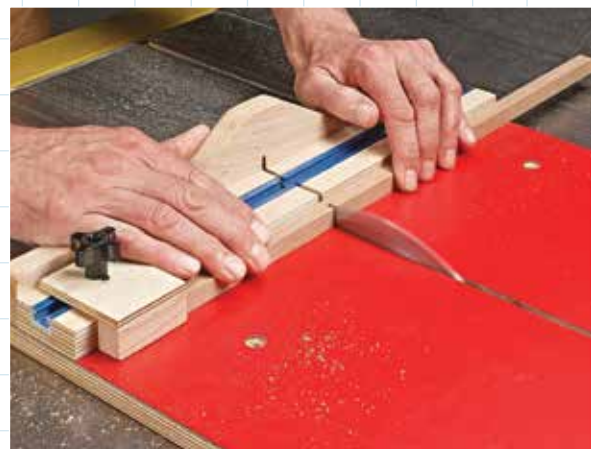
▲ A simple fence with a stop block makes square crosscuts on small parts a sure thing.
