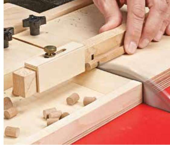
▲ The auxiliary fence platform and tray allow you to cut extra-small parts safely while collecting them in the tray.
